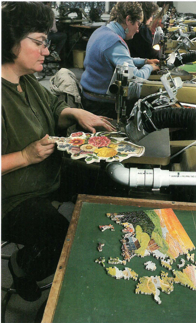
Cutter in Stave's Vermont facility works freehand at a jigsaw with a blade that's as thin as a horse-tail hair.
