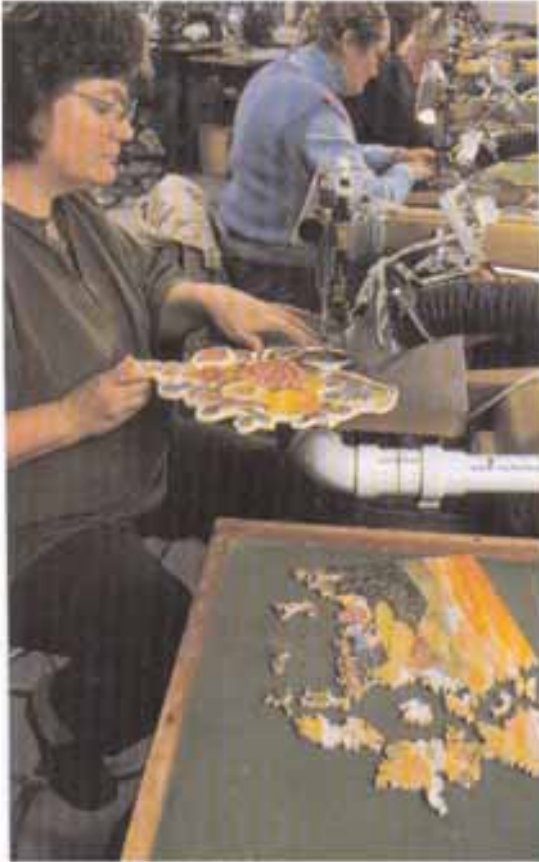
Cutter in Stave's Vermont facility works freehand at a jigsaw with a blade that's as thin as a horse-tail hair.
